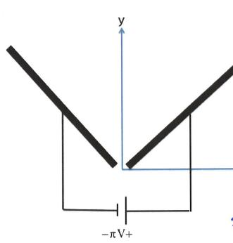
from symmetry the potential is only a function of  $\beta$  with boundary conditions  $V\left(\frac{\pi}{4}\right) = \pi V$   $V\left(\frac{3\pi}{4}\right) = 0$
