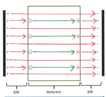
The only free charge is on the plates. So the electric flux density in the gaps and dielectrics will be  $\vec{D} = 5\left(\frac{10}{36\pi}\right) \hat{A}_X \frac{C}{m^2}$ The Polarization is due to bound charge so in the dielectric  $\vec{P} = \left(\frac{10^9}{36\pi}\right) \hat{A}_X \frac{C}{m^2}$
